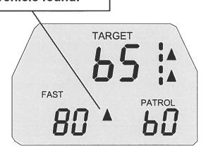
When operating the radar in Same-Direction mode, the same direction road indicator corresponding to the antenna selected will be on solid, and the strongest vehicle speed will be displayed in the TARGET window.
