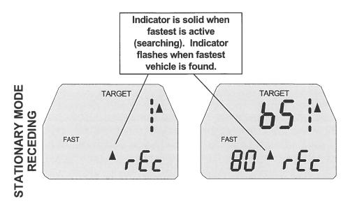
To place the unit in the stationary mode, monitoring receding traffic, repeatedly depress the MODE switch until "rEc" is displayed in the PATROL window.
